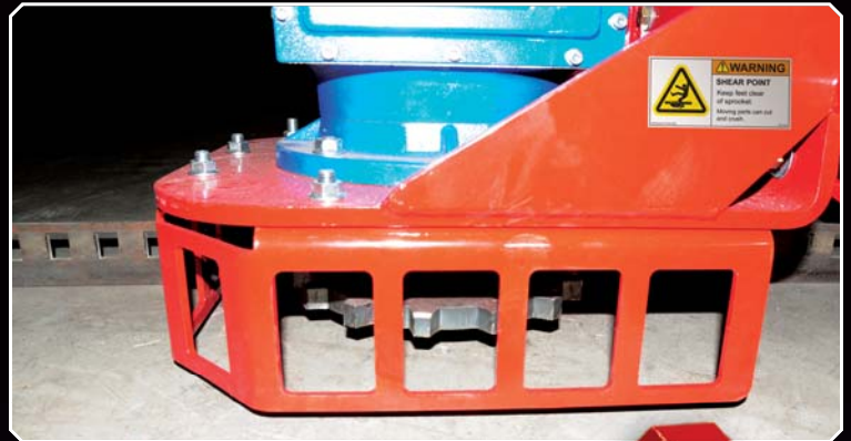
Drive assembly sprocket engaged to track enables forward and reverse travel with no drive slippage.
