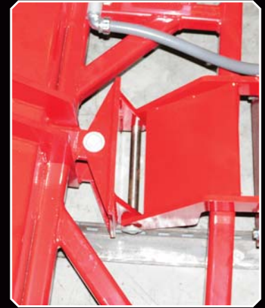
Pivot pin design attaches drive assembly to sweep.
