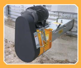
Electric Powerhead with quick detach motor mount and over center belt tensioner. A rubber gasket on the belt guard maintains tube pressurization for a positive airflow seal.
