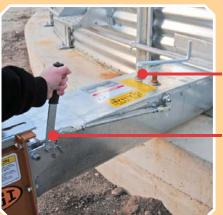
Rack and pinion gate controls are standard on all unloaders.
