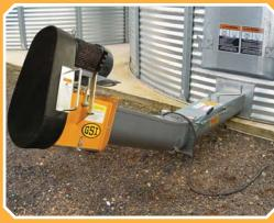
Incline Elbow elevates the discharge to a fixed angle, 20" lift from center discharge to ground.
